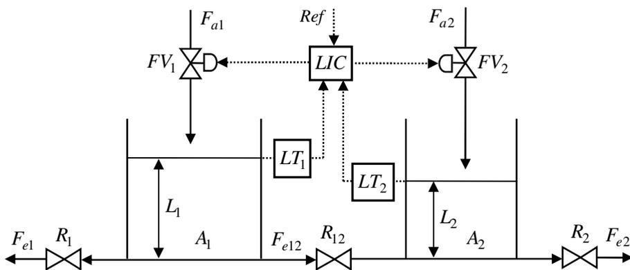
Fig. 1. The scheme of the two coupled tanks.
